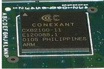
A [Conexant](#) ARM processor used mainly in [routers](#)
